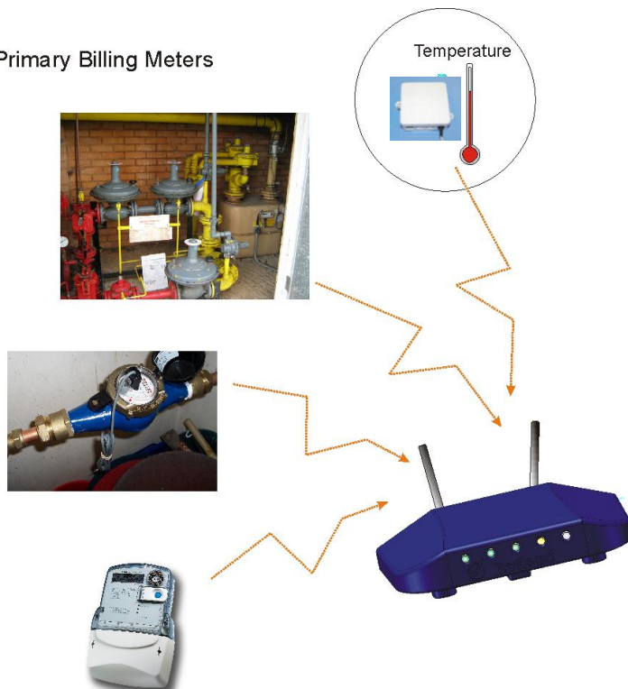
Automated Meter Reading (AMR) for Primary Metering
