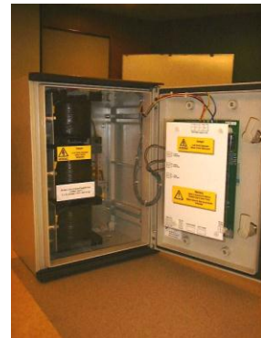
Z-LYNK LPT Controller measuring just 400*300*200 (H*W*D mm)
